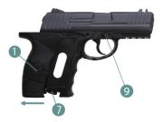
Put the safety on "SAFE" (9) and remove grip cover rearward exposing the CO<sup>2</sup> housing (1).
